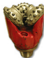
Mall pillow of the drill used to perforate the land
